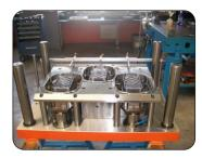
The mould adopts, pneumatic sprint device: die long life, stable quality, high precision, superior design. Aluminium foil container processing from material cut, forming, stretching, curling forming a container shape complete.
